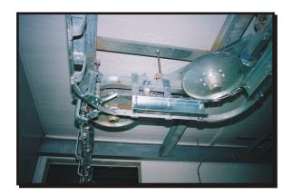
Stainless steel shackles in bleeding conveyor Transfer carcass over bleeding and dressing areas Veterinarian inspector can inspect carcass and offal simultaneously
