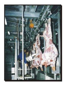
Overhead conveyors, bleeding and dressing Pneumatic feeding and leg spreading device Offal and organ conveyors synchronized with master conveyor Hot dip galvanized track rails, zinc plated chains and chain wheels pneumatic operator lifting platforms
